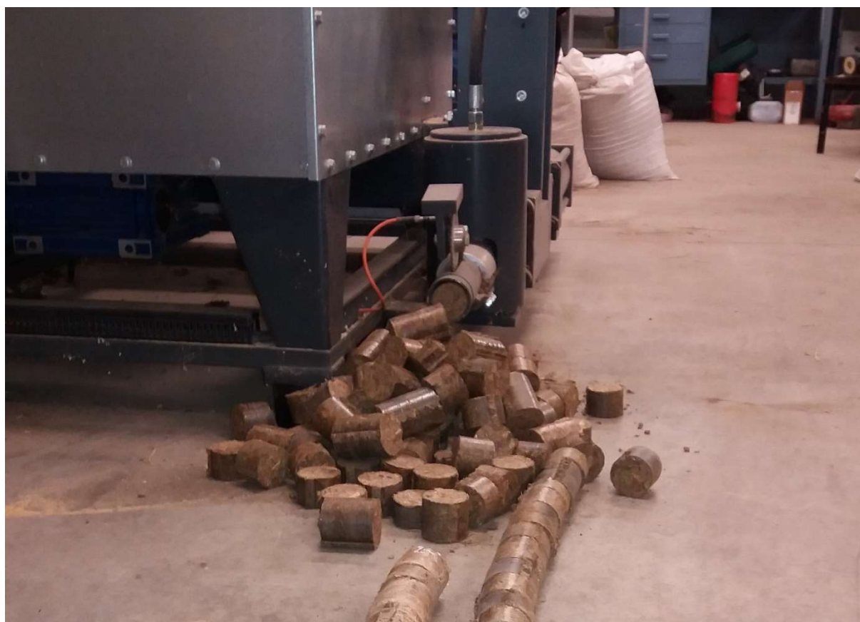
Figure 4. Processing briquette with hydraulic press Weima C-150
